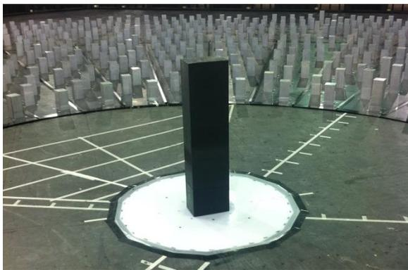
WindEEE can also be used to test large scale, prototype or full scale objects to a wide variety of wind fields. Applications range from testing of full scale solar panels and small wind turbines, large scale topographic and canopy models, large and full scale wind turbine components (blades, towers), building components, environmental measurement devices, unmanned flying vehicles, etc.
