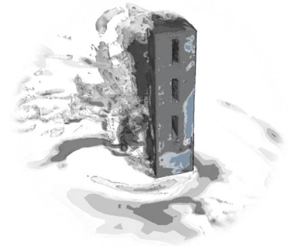
Wind load reduction through use of “openings”
