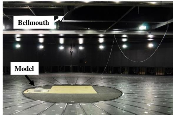
Figure 1. Test setup at the WindEEE dome for one of the offset downburst cases
