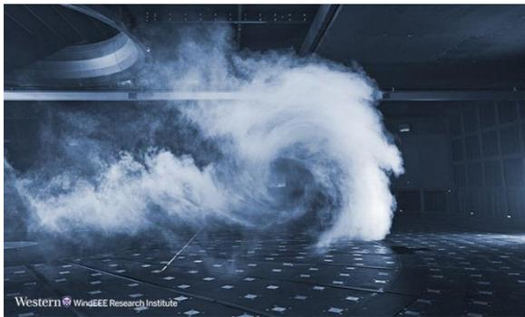
All of WindEEE's different flow configurations can be used to determine pressures and dynamic response of various structures. Scale models of buildings (residential, commercial, industrial, hospital, high-rise), bridges, transmission towers, wind turbines and many others can be tested. Various techniques are used to simulate the effect of surrounding buildings, topography and canopy in order to replicate the local site conditions.
