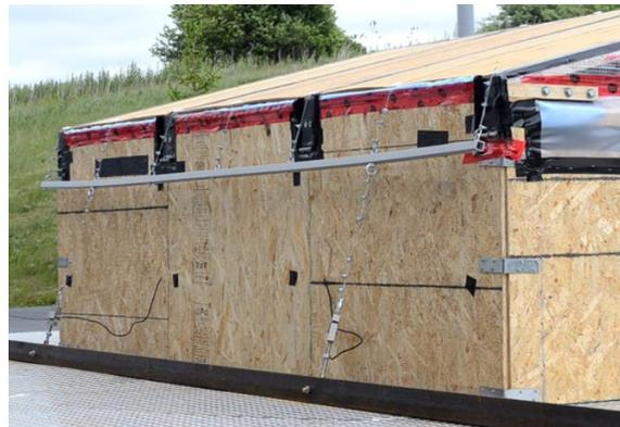
Windward face of the reduced scale retrofitted test specimen on the exterior platform of the WindEEE Dome
